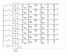
Note: For compatibility reasons the inputs SW\_0 and SW\_1 are to be found on X4-12 and X4-11. If only 8-bits are to be used, SW\_0 and SW\_1 must be on Low (and/or open).
