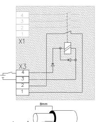
Cable cross section: 0.4 ... 1.5 mm2 (AWG 21 ... 16) single/fine strand
