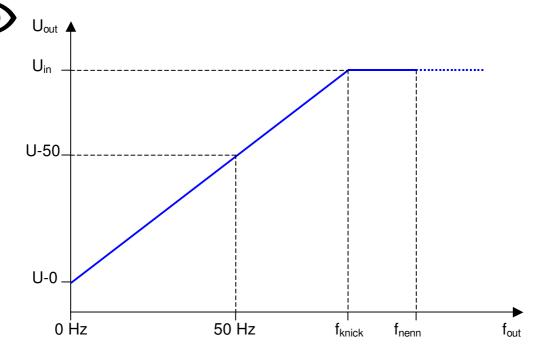
The diagram shows the relationship between output frequency  $(f_{out})$  and output voltage  $(U_{out})$ . The position and steepness of the characteristic curve is determined by the two parameters U-0 (voltage when  $f_{out}=0Hz$ , also termed Boost) and U-50 (voltage when  $f_{out}=50Hz$ , can as a rule be taken from the motor rating plate).
