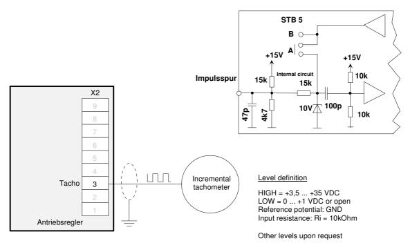
Tacho (X2-3) Pulse-train from incremental tachometer
