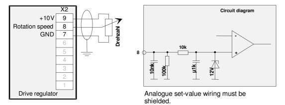
**Speed** (X2-8) Unipolar input for the manual speed-set value specification. This function can be selected with the jumper STB3 "set value source, (see chapter 5.3). Input voltage:  $0 \dots +10$  VDC Input resistance: Ri = 100 k $\Omega$ Reference potential: GND
