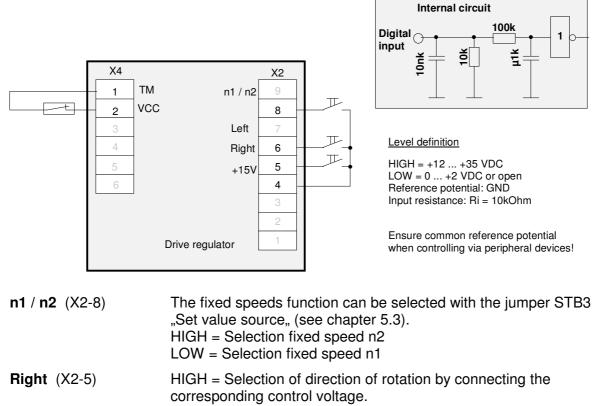
Left (X2-6) If both direction of rotation inputs are selected, the power amplifier remains cut-off.. LOW = power amplifier cut-off
