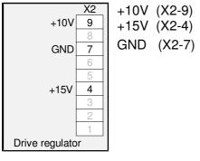
max. load 3 mA (13...17V) max. load 50 mA
